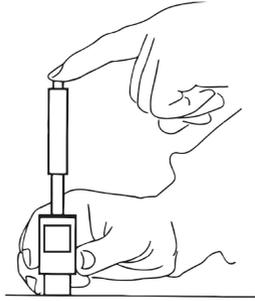
1. Hold the Loading Tube and slide it towards the supporting ring until the impact body is hooked. Then, while still holding on to the Loading Tube, slowly return it to its original position.
